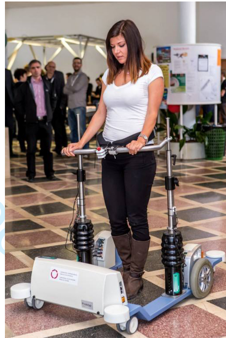
Fig. 3. Hoist system demonstration and testing.
